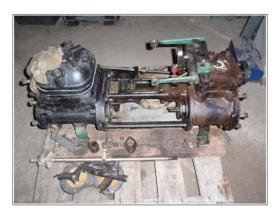
The Northern Plant engine continues to have further work. During the winter it has been protected from the worst of the weather by removable shuttering made by the engineering team. The governor for this engine was removed, dismantled and cleaned by shot blasting. The frame was painted by the powder coating technique and the other parts spray painted before reinstallation (pictured).
